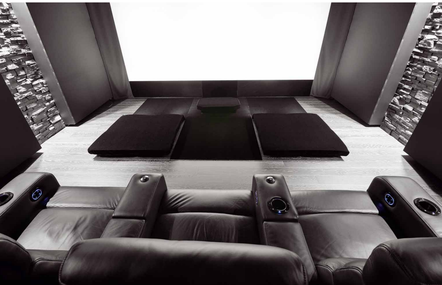
No sunbathing lawn: Directly in front of the screen, these absorbers are designed to eliminate the initial reflection from the lower center speaker to the listening position
