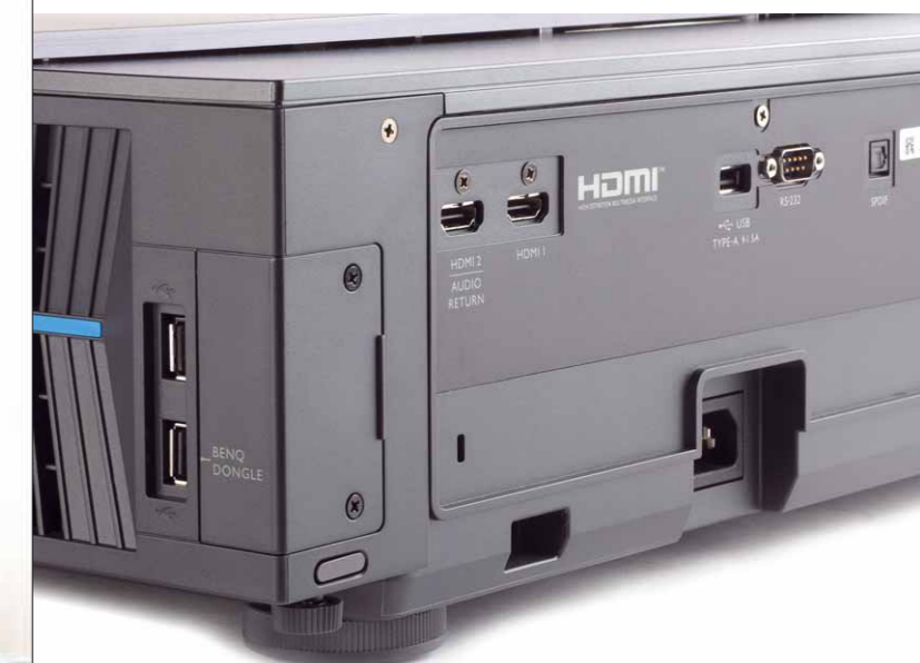
Two HDMI inputs on the back are available for conventional sources; the two USB sockets on the side are responsible for external media or the optional WiFi dongle.
