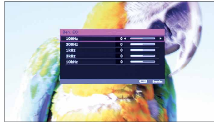
In the user menu, the sound can be individually adjusted with the help of a 5-band equalizer
