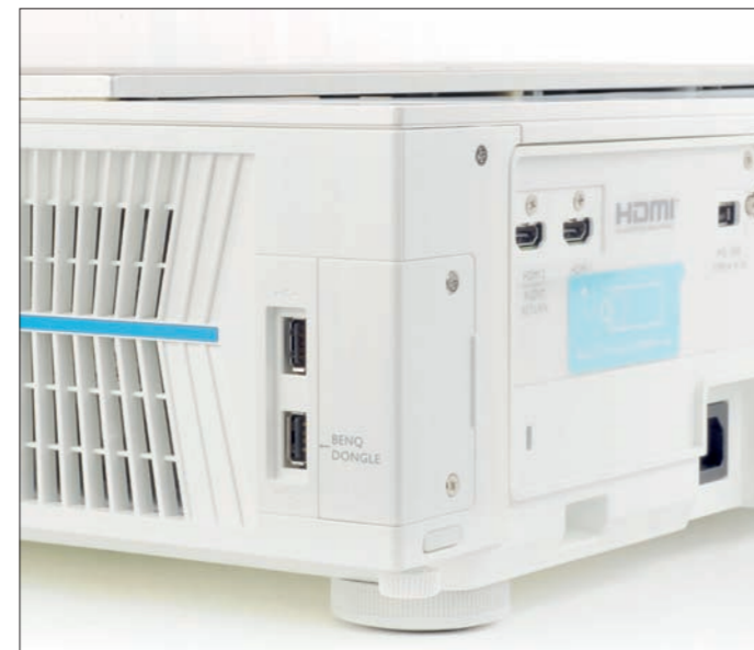
Even with the dongle inserted, two more USB interfaces are available for the integrated media player
