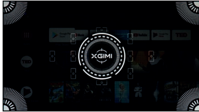
Immediately after switching on or when the projector has been moved, it automatically refocuses the image via autofocus
