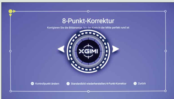
The projector focuses automatically. The keystone correction can also be corrected manually at a total of eight individual points
